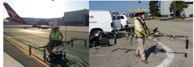
Fig. 4. Mounted Gradiometric Receiver Instrumentation.
